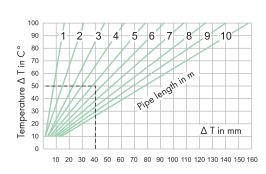
This table provides graphic determination of expansion at known pipe length at a change of temperature in the pipeline.
